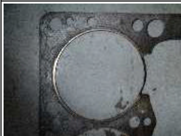
(5) Passenger-Side Head Gasket: #8 Blown (Fire Ring was crushed at top of cylinder - misalignment)
