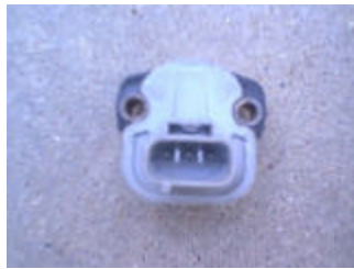
Factory TPS Sensor w/Brass Inserts
