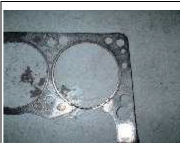
(1) Passenger-Side Head Gasket: Blown cylinder (4-5# boost) - Notice O-Ring impression - Misaligned
