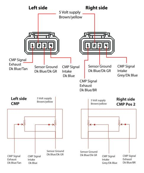
Next, measure the resistance in the CMP connector between the supply voltage terminal and the ground terminal. If the resistance
